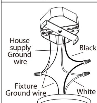
3. Connect the ground wires (bare copper or green) from your fixture to the ground wire (bare copper or green) or ground screw in the electrical box. Attach the black wire from the light fixture to the black wire in the electrical box. Attach the white wire from the light fixture to the white wire in the electrical box.
