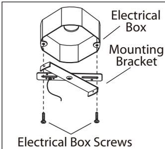
1. Mount the mounting bracket to electrical box using electrical box screws (not included).
