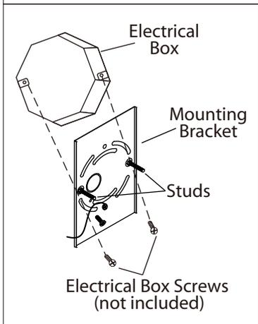
2. Mount the mounting bracket to electrical box using electrical box screws (not included). Make sure the studs on the mounting bracket are facing out from the electrical box.
