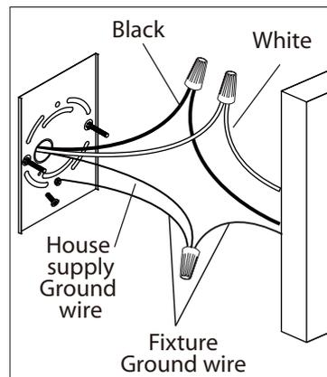
3. Connect the ground wires (bare copper or green) from your fixture to the ground wire (bare copper or green) or ground screw in the electrical box. Attach the black wire from the light fixture to the black wire in the electrical box. Attach the white wire from the light fixture to the white wire in the electrical box.
