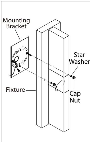
1. Remove the mounting bracket from the fixture by unscrewing the 2 cap nuts.
