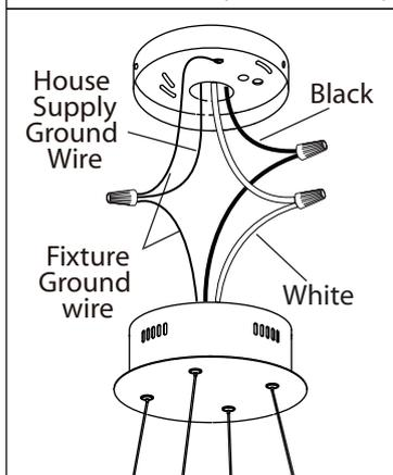
2. Connect the ground wires (bare copper or green) from your fixture to the ground wire (bare copper or green) or ground screw in the electrical box. Connect the black wire from the fixture to the black wire in the electrical box and connect the white wire from the fixture to the white wire in the electrical box.
