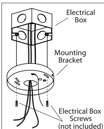
1. Feed power cords from the electrical box through the centre hole of the mounting bracket. Mount the mounting bracket to electrical box using electrical box screws (not included).
