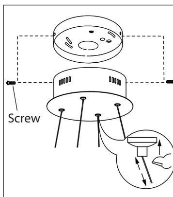
3. Attached fixture to mounting bracket by tightening the 2 screws.
