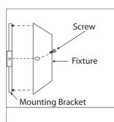
4。Attached fixture to mounting bracket by tightening the 2 screws.
