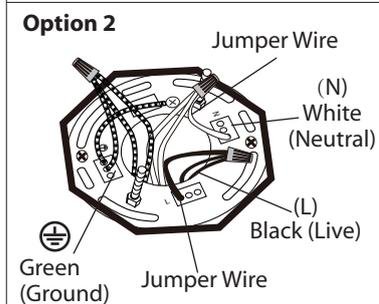
2. **Option 2:** For multiple green (ground), black (live) and white (neutral) wires joined in the electrical box (house wiring), attach a single "green", "black" and "white" jumper wire before connecting. Strip 7mm from the 6" jumper wires (AWG 12-24) supplied. Then connect (push) wires into the correct inserts.
