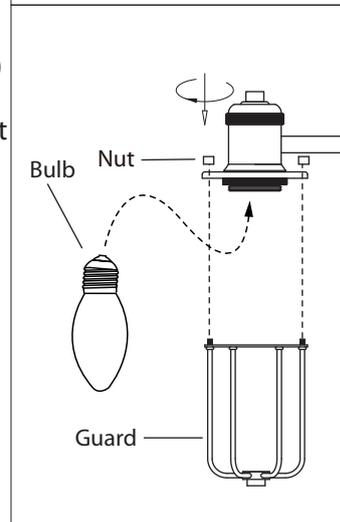
5. Unscrew the nuts to remove the guards.
