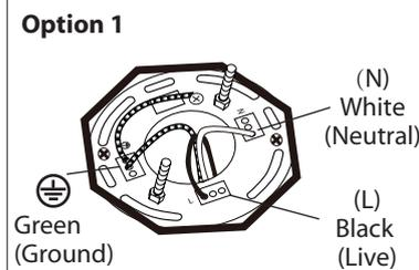
2. **Option 1:** Connect (push) electrical wires from electric box (house wiring) into correct inserts.
