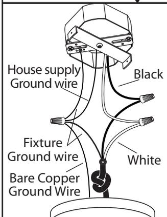
3. Connect the ground wires (bare copper or green) from your fixture to the ground wire (bare copper or green) or ground screw in the electrical box. Connect the black wire from the fixture to the black wire in the electrical box and connect the white wire from the fixture to the white wire in the electrical box.
