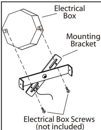
1. Mount the mounting bracket to electrical box using electrical box screws (not included).
