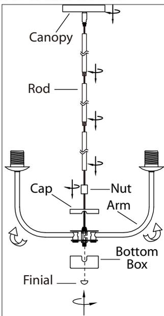
1. Spread the arms evenly. Tighten the bottom box with the finial against the stud. Tighten the cap against the assembly by the nut.
